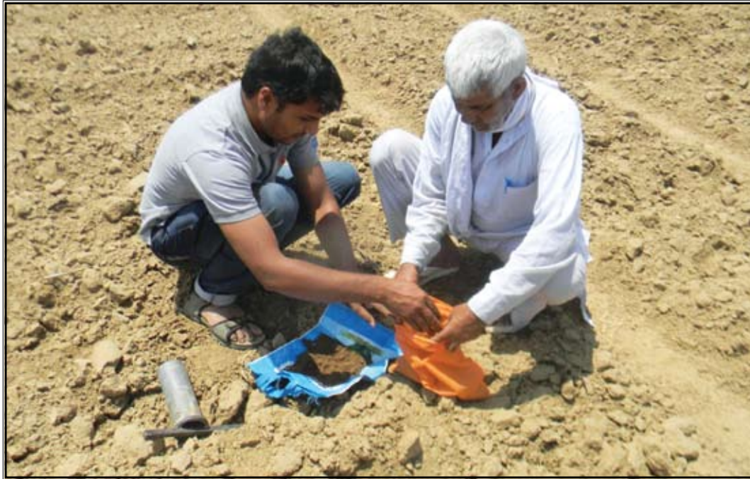
Figure 17: Proper collection and labelling of the soil samples and field testing for critical nutrients
